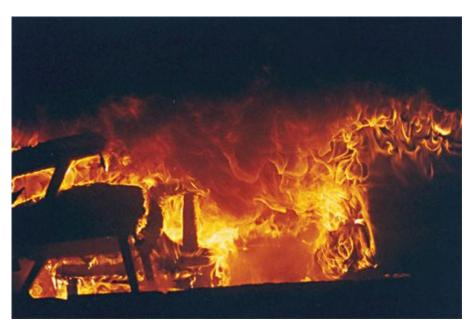
(5) Thermal collapse shown post-flashover in the flashover simulator.
