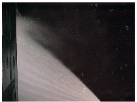
(4) This fog stream is being directed into a room that is vented with a three-foot × seven-foot oversize door. It is moving approximately 5,000 cubic feet of air per minute into the room, overpressurizing the room. The steam is being driven onto the attack crew.
